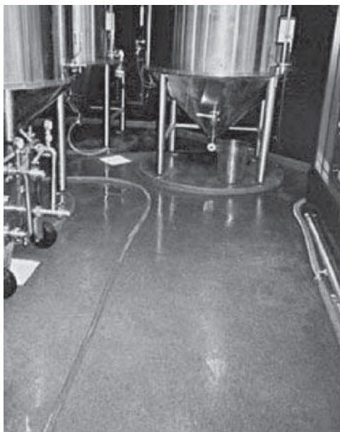
FIGURE 11 The process area is subjected to substantial chemical action due to the sterilizing protocol. It has a troweled epoxy, easy-to-clean finish. (Courtesy of Dex-O-Tex.)
