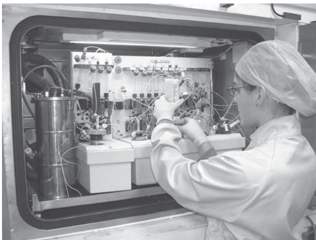
FIGURE 7 Automated synthesis module for PET radiopharmaceutical synthesis located in a shielded hot cell. (Photo courtesy of PET-CUN Center, University of Navarra.)
